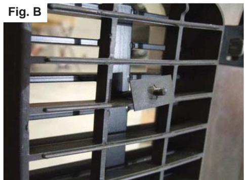
**Step 3:** Turn the bolt so that the speed nut is perpendicular to the horizontal bars in the grille **as shown in fig.C.** Pull out on the billet grille so that there is pressure on the speed clip. This will hold the speed clip in position and allow you to finish tightening the bolt into the speed clip.
