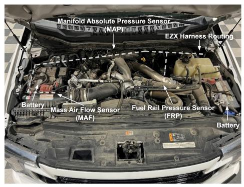
**STEP 2** - Locate the MAF connector on the intake box, and disconnect it by pulling the locking tab up then squeeze the release tab. Connect both connectors to the EZX harness.
