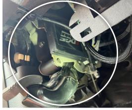
**STEP 16 -** Use the provided zip ties to secure the excess cable from touching hot surfaces or any moving components.
