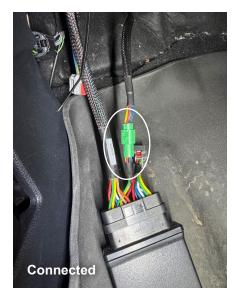
**STEP 8** - Locate the APP Sensor above the accelerator pedal and disconnect it by pulling up on the red locking tab and then pushing in the release tab. Connect both connectors to the EZX harness.
