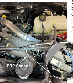
**STEP 4** - Locate the FRP Sensor by the coolant reservoir, and disconnect it by first pulling the lock tab out, then by squeezing the release tab. Connect both connectors to the EZX harness.
