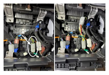
**STEP 13 -** Once cable is routed and secured as shown previously, reinstall the glove box.
