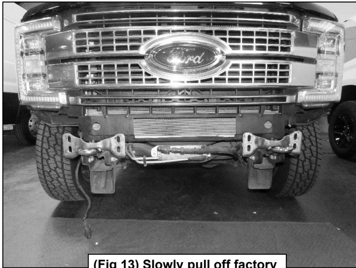
(Fig 13) Slowly pull off factory Front Bumper with help.
