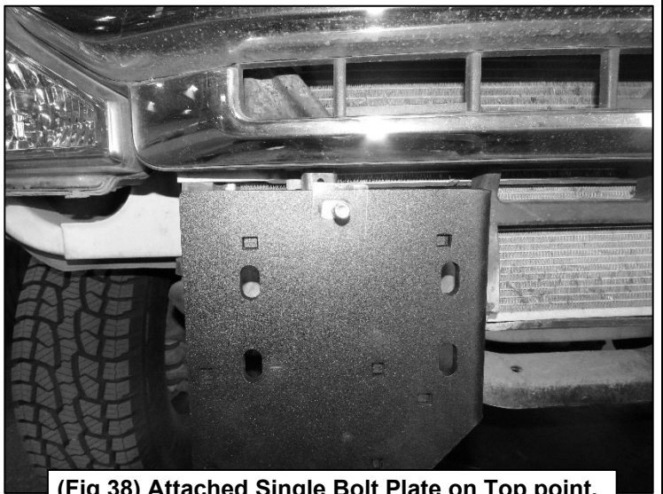
(Fig 38) Attached Single Bolt Plate on Top point.
