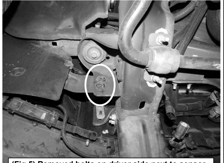
(Fig 5) Removed bolts on driver side next to sensor.
