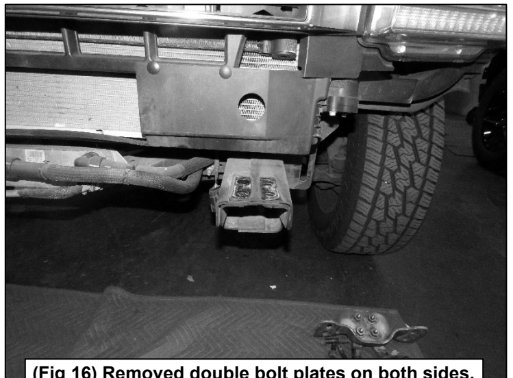
(Fig 16) Removed double bolt plates on both sides.
