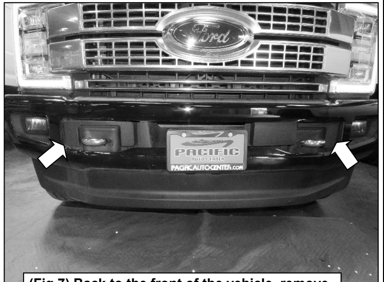
(Fig 7) Back to the front of the vehicle, remove plastic covers to remove bolts.
