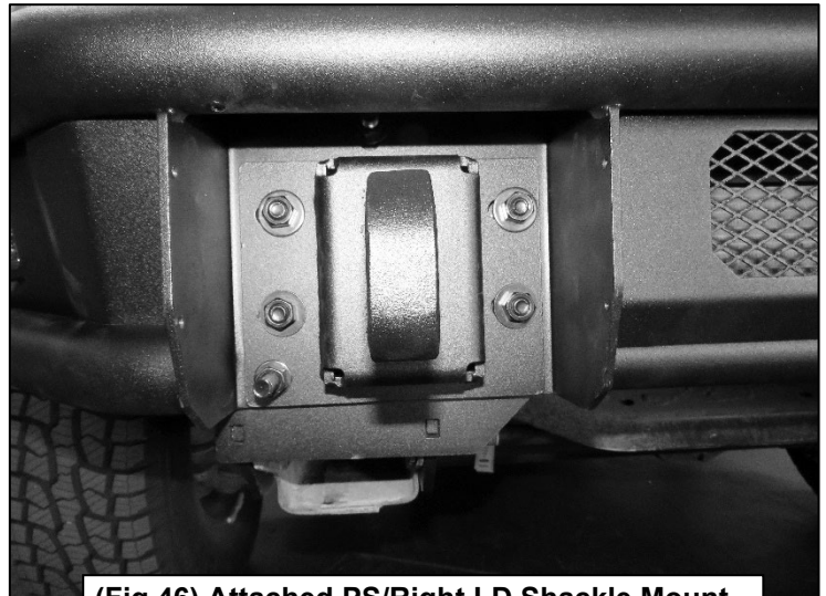
(Fig 46) Attached PS/Right LD Shackle Mount.
