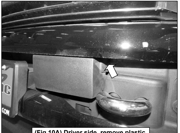
(Fig 10A) Driver side, remove plastic cover bolts to relocate ACC sensor.
