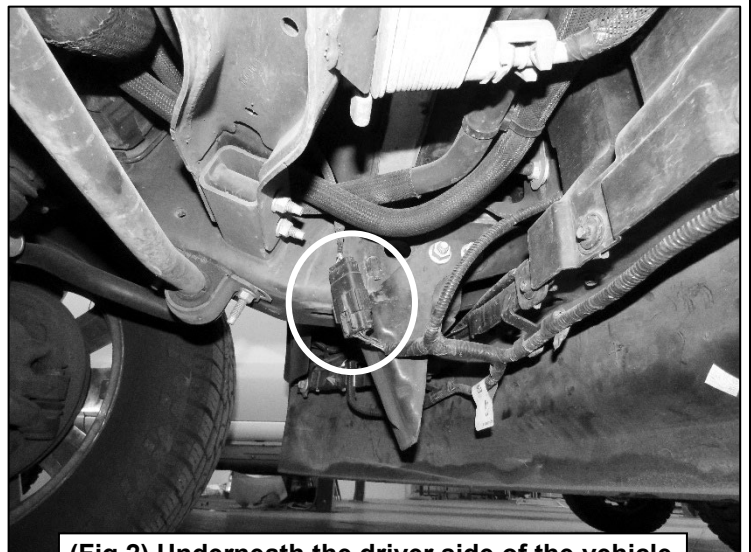
(Fig 2) Underneath the driver side of the vehicle unplug sensor for front bumper removal
