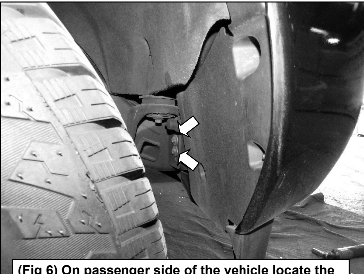
(Fig 6) On passenger side of the vehicle locate the same bolts to remove for front bumper removal.
