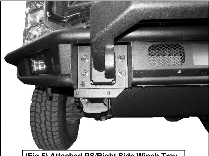
(Fig 5) Attached PS/Right Side Winch Tray.
