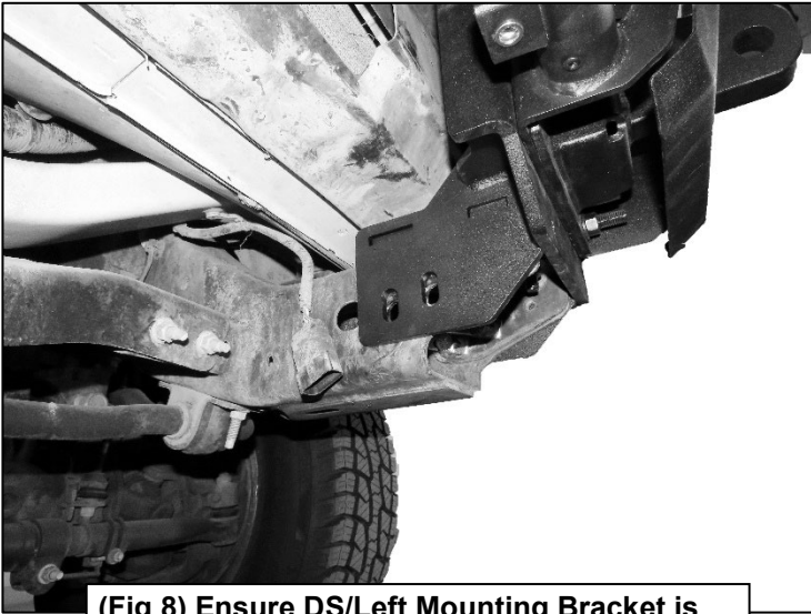
(Fig 8) Ensure DS/Left Mounting Bracket is aligned to mounting points on frame.
