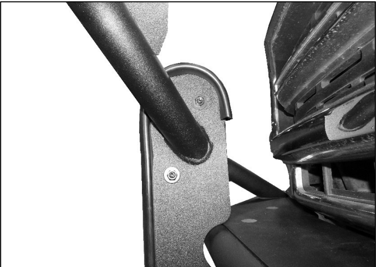
(Fig 8A) Attached PS/Right Wing Guard Tube onto HD4 Push Bar and repeat for DS/Left Wing Guard Tube.
