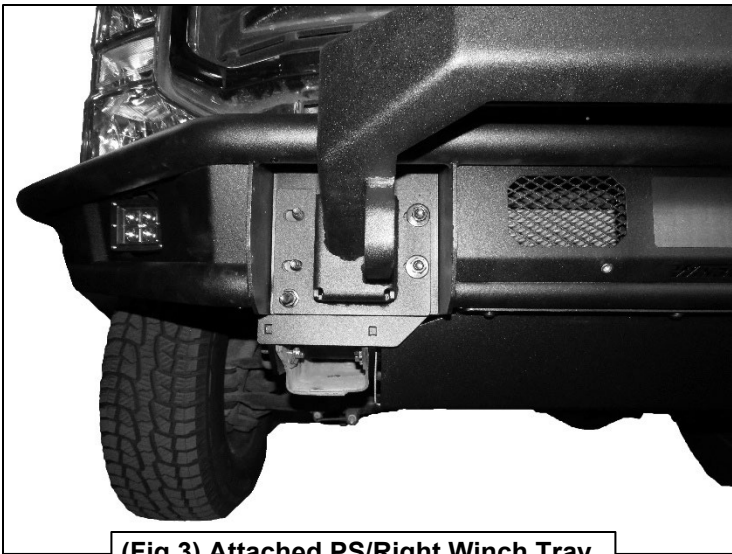
(Fig 3) Attached PS/Right Winch Tray.
