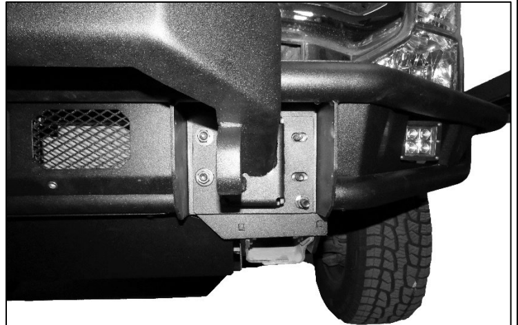
(Fig 4) Attached DS/Left Winch Tray.
