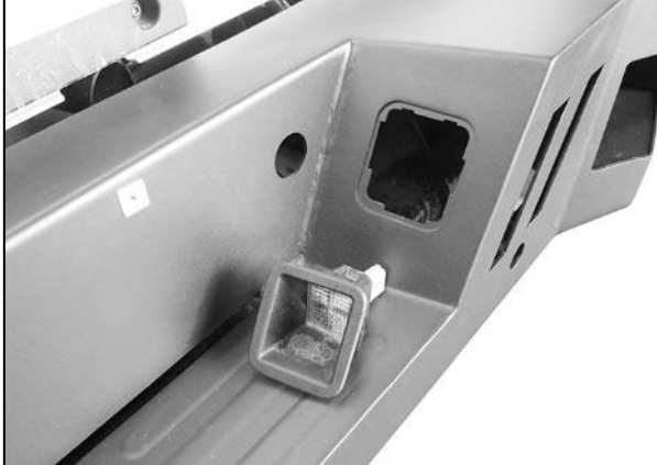
(Fig 17) Push license plate lights into openings and plug into bumper wiring harness
