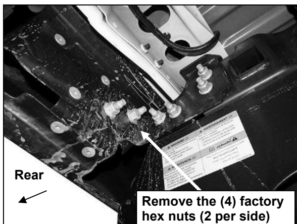
(Fig 3) Remove hex nuts to remove bumper assembly. 2017-22 model pictured
