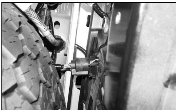
(Fig 1) Unplug and move all wiring harnesses away from bumper. Trailer plug pictured
