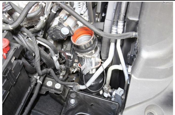
18. Insert the HPS charge pipe #1 into the charge pipe #2 until the coupler hits the sensor bracket.
