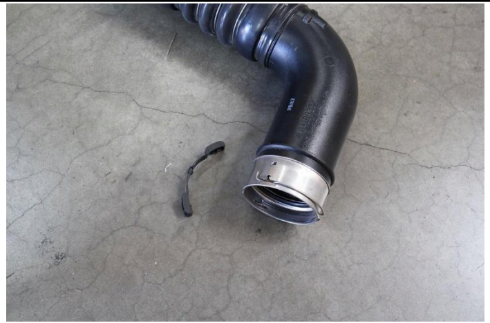
16. Once the plastic clip is removed you can now remove the metal retaining clip from the stock charge pipe.
