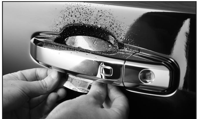
**1** Spray slip solution on the door cup area, fingers and protection film before and as the film is removed from the backing.
