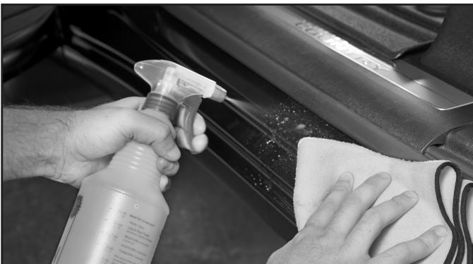
**3** Thoroughly clean all areas with prep/tack solution to remove any dirt, debris, grease or oil. Dry with a clean, lint-free cloth.
