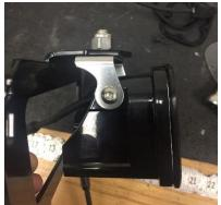
4. Install the Baja Designs Brackets and Lights into the OEM location using the factory 10mm bolts.
