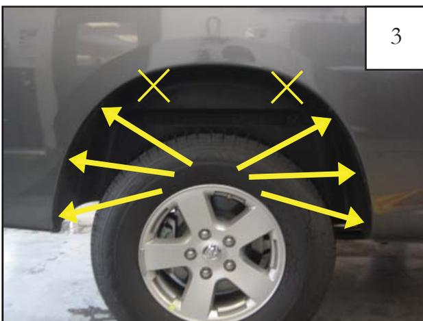
Remove six factory installed screws using an 8 mm socket wrench. X's indicate a factory screw that will not be removed.
