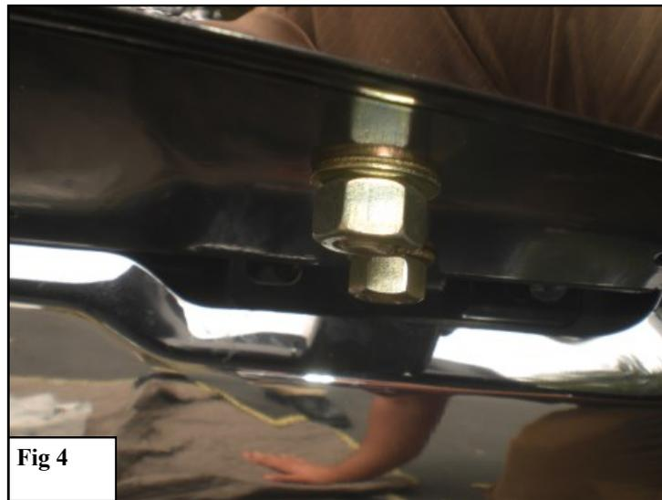
5. Align and adjust the winch tray as needed then fully tighten all hardware at this time. Torque all M12 hardware to 50-55 ft lbs and M10 to 40-45 ft lbs.
