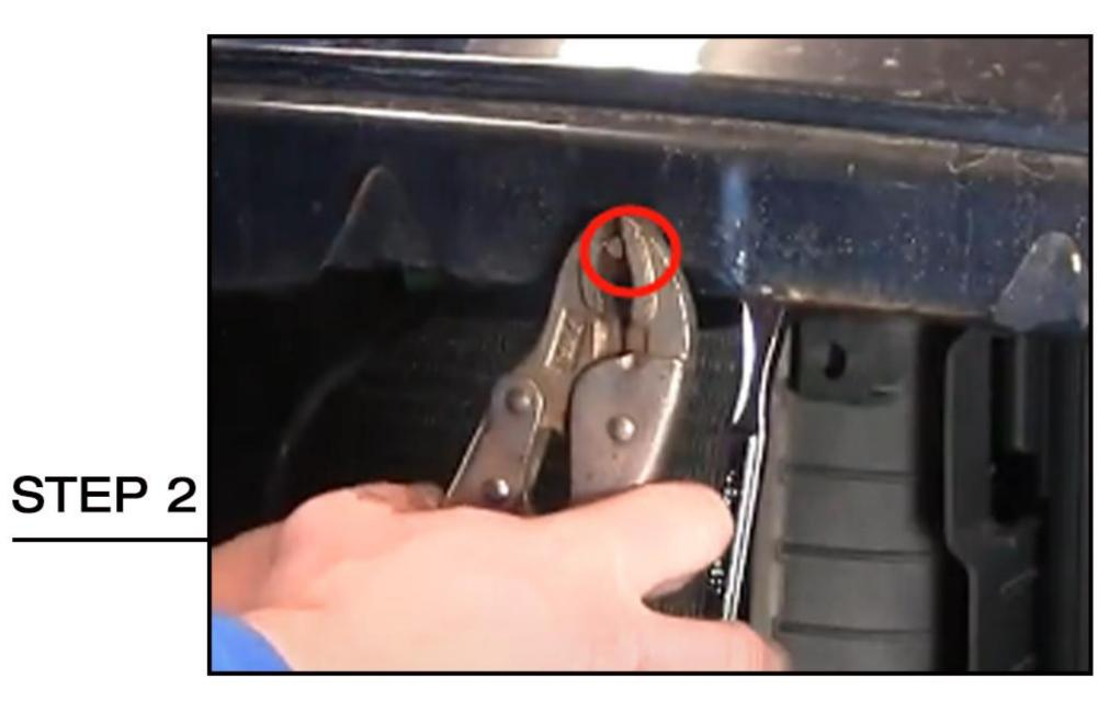
Remove all the metals from the plastic and metal nuts that are on the back with a pair of vice to save the nuts for the new grille. (You can clean the surface and put a coat of wax)
