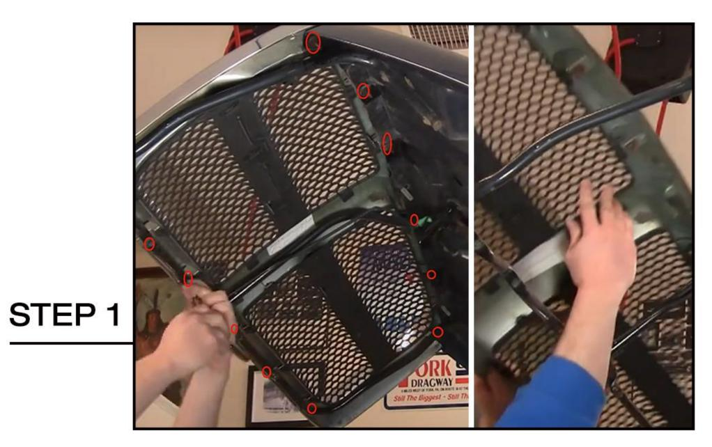
Open the hood,remove 12 bolts(6 on each side) with 8 mm socket ratchet to remove the old grille.
