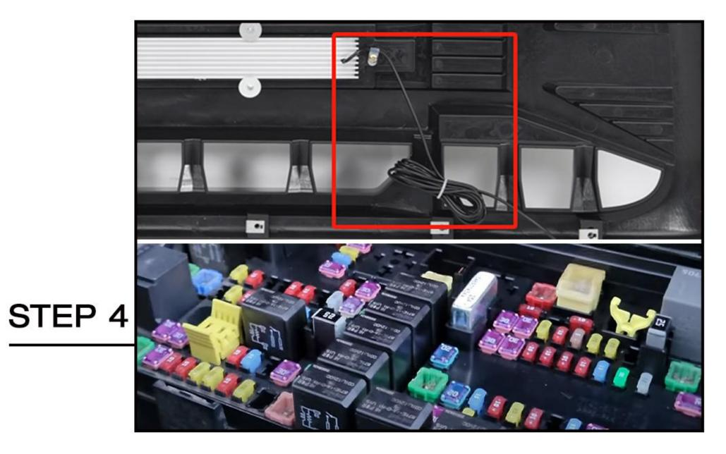
DRL Wiring: Wire to fuse box, the red wire connects to the ACC, the black wire connects to the negative of battery.
