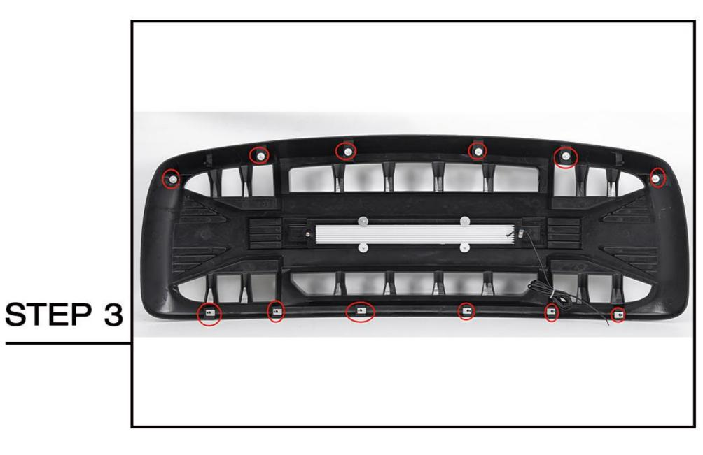
Align the top 6 screws on the back of the new grille and the bottom 6 metal clips (installed on the grille, not separately equipped with screws) with the holes on the body of the vehicle.
