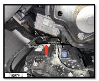
**Step-1** Open the hood and disconnect the vehicle battery. Beginning on the driver side, go under the vehicle and if equipped disconnect the factory fog light wiring harness from the fog light (FIGURE 1).
