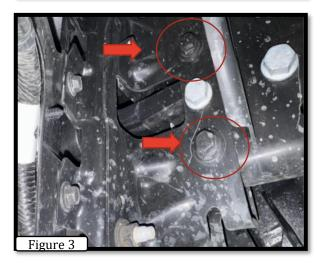
**Step-3** Remove the bolts(2) per side and nuts securing the bumper brackets to the frame using an 18mm socket and ratchet. With assistance remove the factory bumper from the vehicle and set it aside. (FIGURE 3). Repeat Steps on passenger side.
