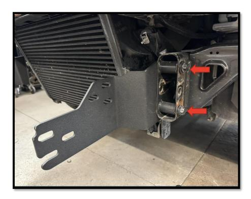
Step-1 Install the driver side frame bracket by positioning the bracket on the inboard side of the frame. Align the holes in the frame bracket with the holes in the frame used for the OEM bumper bracket attachment, and then secure the bracket to the frame using the ½'X 3 ½" Hex bolt (2) ½" Hex Nut (2), ½" Flat Washer (4), ½" Lock Washer (2), (Fig 1 & 2). Leave the nuts and paired bolts loose for final adjustment. Repeat this step to install the passenger side frame bracket.
