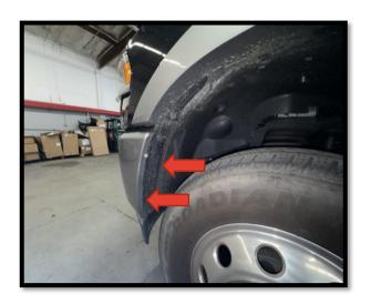
**Step-4** Use the appropriate pry tool to pull the inner fender liner out from the outer bumper. With assistance remove the factory bumper from the vehicle and set it aside
