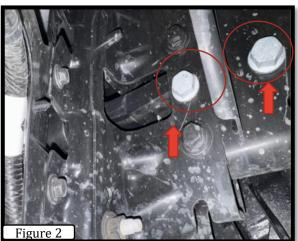
**Step-2** Remove the nuts and bolts (2) per side securing the factory tow hooks to the frame using a 24mm wrench, socket and ratchet, (FIGURE 2). Repeat Steps on passenger side.
