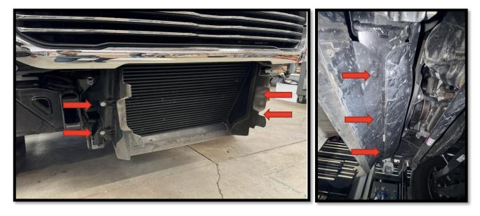
**Step-5** Remove the (4) bolts using a 10MM socket and (3) plastic push in connectors securing the shroud to the bottom of the intercooler using the tip of a screwdriver. **You may reinstall the intercooler shroud once the winch tray is installed. Using the appropriate cutting tool, trim the sides to fit accordingly.**
