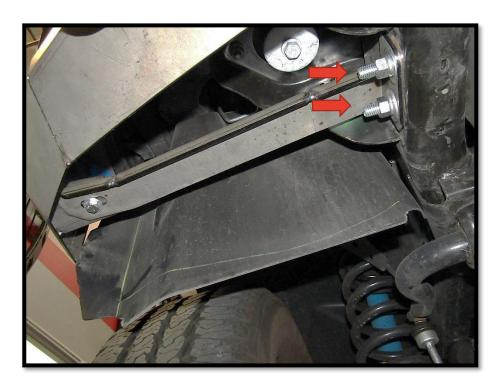
*Step-6* Attach the opposite end of each support bracket to the bumper shell bracket using (1) 1/2" x 1 1/2" hex bolt, (2) 1/2" flat washers, (1) 1/2" lock washer and (1) 1/2" hex nut, (Fig 10). Trim the fender liner to your desired fit with the appropriate cutting tool.
