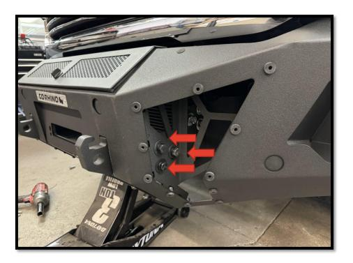
Step-5 With assistance lift the bumper shell up to the vehicle, align the holes in the bumper shell brackets with the holes in the frame brackets, and weld nuts on the winch tray. Secure the bumper shell bracket to each side of the winch tray using (3) ½" x 1 1/2" hex bolts, (3) ½" lock washers and (3) ½" flat washers, (Fig 9). Leave the bolts loose for final adjustment.
