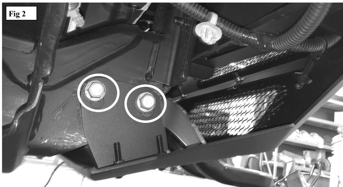
3. Install mounting brackets items 2 and 3 on frame according to **Figure 2** using M12 hardware (**Items 4-7**).
