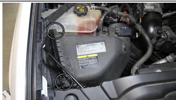
5. Loosen the two bolts securing the upper air box assembly.
