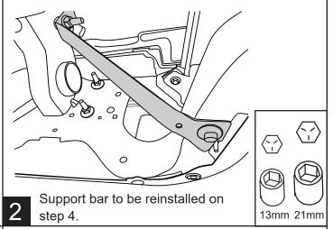
Remove 2 nuts and set assembly into position. Reuse factory nuts and Torque to 41ft-lbs/ 55Nm.
