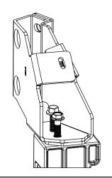
Remove support bar with a 21mm deep socket and a 13mm socket or wrench.
