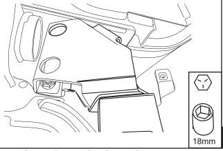
Replace support bar and slide support strap over stud. Use supplied hardware to bolt strap to assembly. Torque to 41ft-lbs/ 55Nm.
