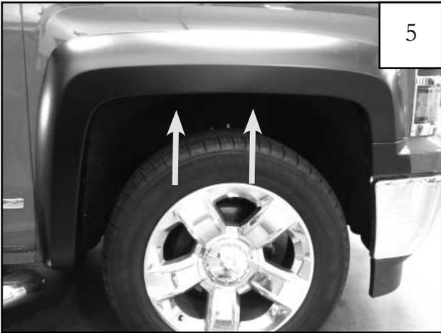
To mount the flare into position, hold the flare 2-3" inches below the top lip of the wheel well. Push in and slide up to allow the flare to fully seat against the wheel well opening.
