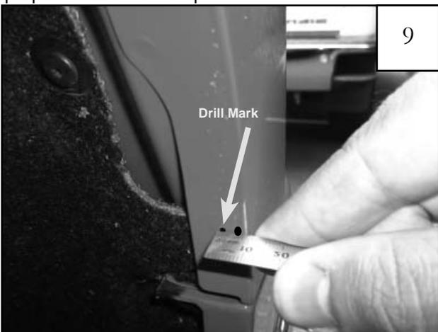
Remove the flare. Using the marks made in step 7 as a guide, measure inward from the outside edge of the fender to verify proper depth of original marked location. Mark must be minimum of 10mm in from outside edge of fender, if short, adjust mark to 10mm.
