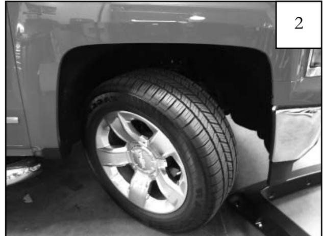
Turn front tire outward for easier installation.
