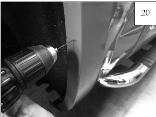
Using a 3/32" drill bit, drill pilot holes at the marks made in Step 19.
