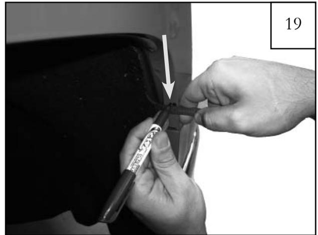
Remove the flare. At the marked locations made in Step 17, measure inward 22mm from the edge of the fender and mark with grease pencil or marker. These are the marks to be drilled.
