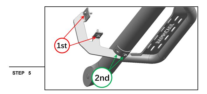
Tighten the mounting brackets to the vehicle. Adjust the side step to the desired angle, and tighten the M8 combo bolts to secure the step into place. See photo for tightening order visual.
