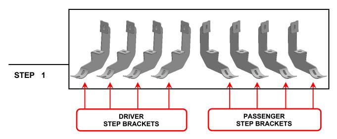
Identify each mounting bracket referencing the diagram above. Notice: The brackets can be used at any position along the same side of the vehicle.
