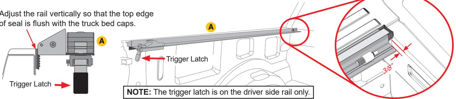
**5** Begin clamping the driver side rail (A) to the truck bed. Start in the middle and evenly space 3 clamps (D) along the rail. You should leave approximately 8" on each end of the rail. Finger tighten the clamps, making sure the teeth properly engage with the grooves of the side rail. Then tighten all clamps with a 1/2" socket or wrench. Repeat step 5-6 on the passenger side rail (B).
