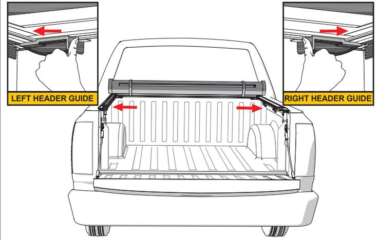
**11** To drive with the cover in the closed position, engage the retainer hooks from the retainer loops and unroll the cover towards the tailgate.
