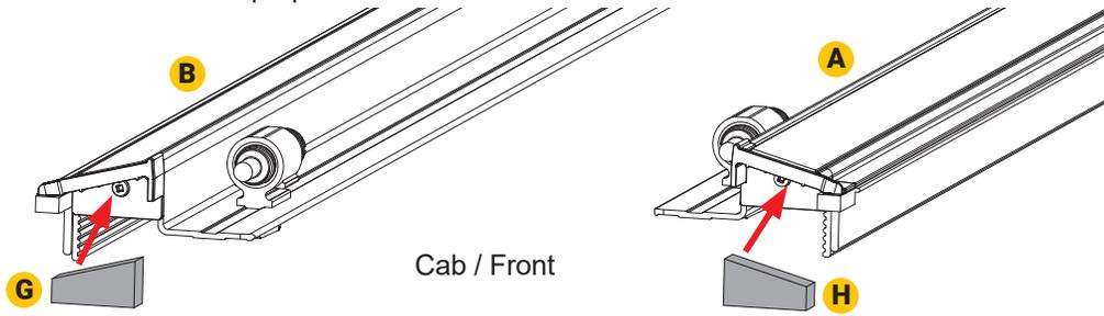
**4** Position the driver side rail (A) to the inside of the truck's bed rail, making sure the flange of the driver side rail fits on top of the bed cap. The front edge of the rails will be 3/8" back from the bulkhead.
