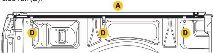
**NOTE:** The use of spring clamps to hold the side rail in place can assist during the installation process.
