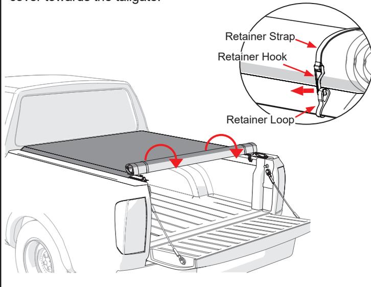
**12** Place the rear header into the header stops which are located on both side rails. Rotate the rear header downwards until you feel the cover latch in place. A clicking sound will indicate a correctly installed cover.
