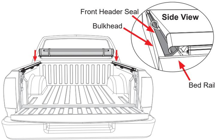
**10** To connect the cover assembly (C) to the side rails (A and B), slide the right and left header guides into the locked position. A clicking sound will indicate a secure attachment.
