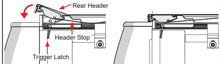
**Preferred method of closure:** Close tailgate, then close cover on top of the tailgate. This method will not work with some truck applications. Use the alternative method instead.
