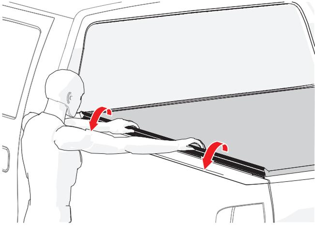
**14** With both sides of the hook and loop engaged, use the palms of your hand to firmly push the loop strip into the hook track. Do this to both driver and passenger sides. **You are ready to drive with the cover in the closed position.**
