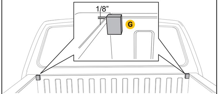
**3** Install end plug seals (G & H) included with cover (A) by cleaning the front of the side rails (A & B) with soap and water to remove dirt and debris. Clean the area with isopropyl alcohol to remove wax or grease and to evaporate any remaining water. Allow the surface to dry. Peel the white paper backing and adhere the seals to the front of the side rails (A & B) as shown. Apply pressure evenly to the entire seal to ensure proper adhesion.
