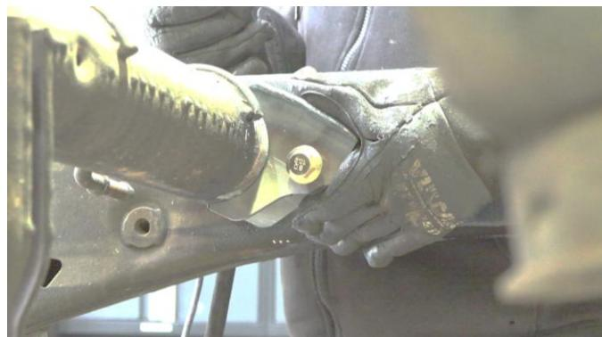
Following proper welding procedures, tac weld your rear shock mount onto the frame before welding it on fully. Weld 100% around all edges.
