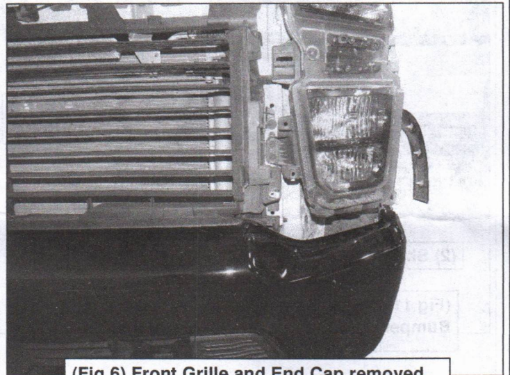
(Fig 6) Front Grille and End Cap removed.
