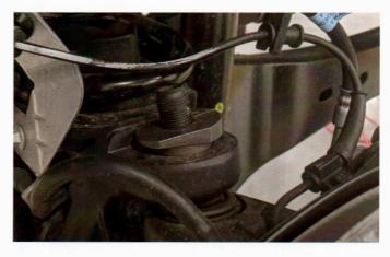
7. Re-install factory castle nut. Torque to factory specs. Ensure there is alignment between castellations on nut and the hole in the ball joint.
