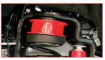
Install the ReadyLIFT sway bar drops to the frame using factory hardware. Torque to 35 ft-lbs. Install the sway bar to the ReadyLIFT sway bar drops using the 7/16" x 1 1/2" bolts, washers and nuts. Torque to 35 ft-lbs.
