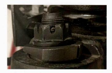
8. Re-insert factory cotter pin into the ball joint and castle nut.
