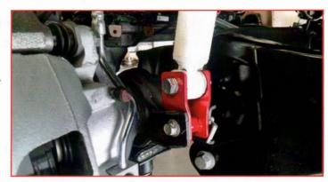
Install the ReadyLIFT brake line bracket to the factory brake line using 5/16" x .75" bolts, washers, and nuts. Install the bolt facing outwards. Gently pull the metal brake line down while lining up the ReadyLIFT bracket to the original holes in the frame. Install using factory hardware. Reattach the brake line bracket at the axle using factory hardware. Torque all to 5 ft-lbs.
