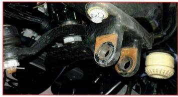
Install the ReadyLIFT track bar bracket to the frame using factory hardware. Torque to 95 ft-lbs. Install the track bar to the ReadyLIFT bracket using factory hardware. Torque the track bar hardware to 250 ft-lbs.
