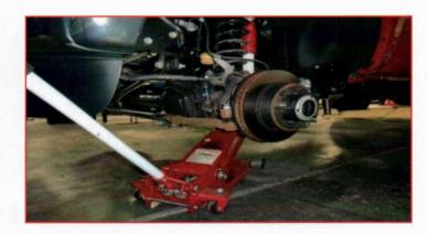
Remove the brake line bracket at the frame.
