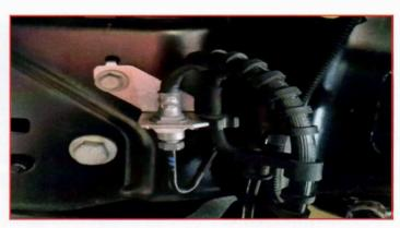
Remove the brake line bracket at the axle.
