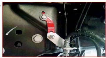
Remove the factory bump stop by pulling it out of its mount. Remove the mount from the frame.
