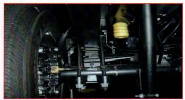
Slightly loosen but do not remove the passenger side u-bolts. Remove the driver side u-bolts completely and discard.
