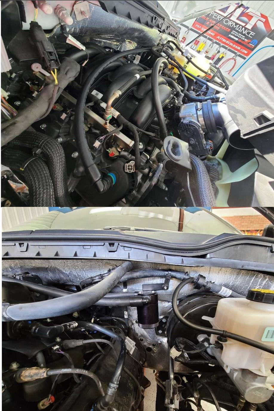
To properly clean the filter in the Oil Separator, spray any degreaser or solvent through it and let it air dry. Clean it every 10,000 miles.
