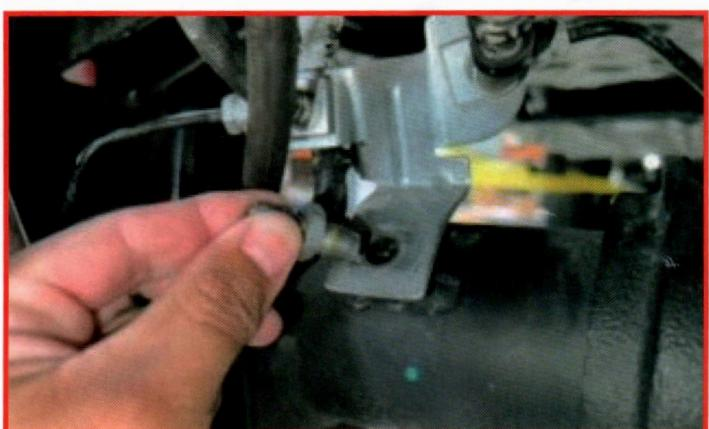
Remove the shocks on both sides of the vehicle.
