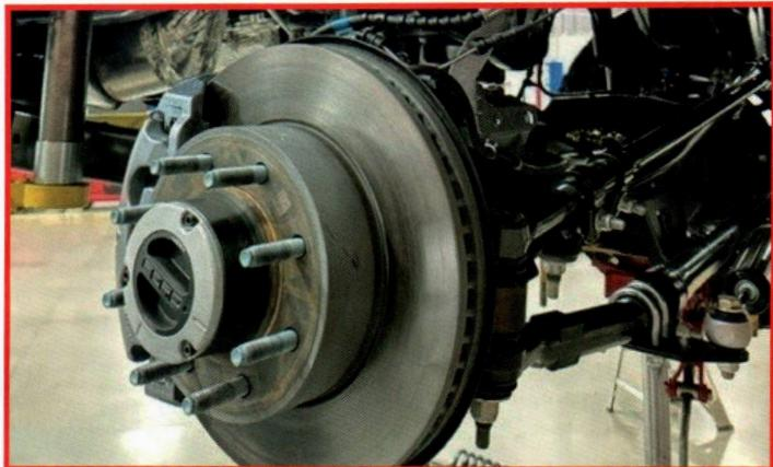
Remove the sway bar from the frame mounts, frame brake line bracket and OE shocks. (both sides).
