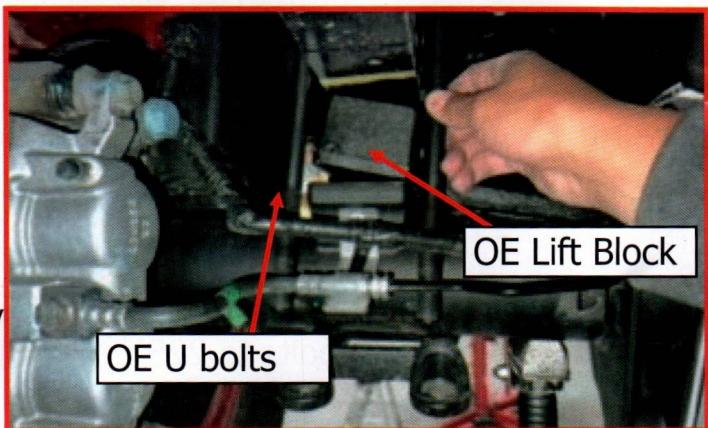
Install the supplied lift block. Use your floor jack to raise the axle to the spring making sure the pin on the factory leaf spring assembly fits into the hole on the lift block. Install the supplied U-bolts, washers and hi-nuts.
