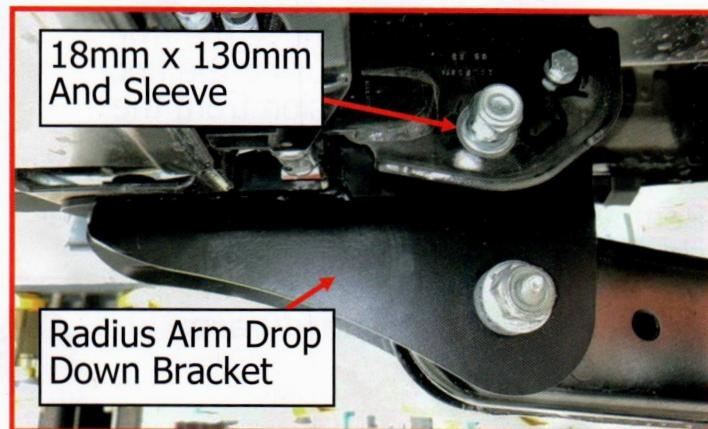
Slide the nut plate, into the frame. Using the supplied **18mm X 40mm bolts, washer and split washer**, Install the bolt through the radius arm drop bracket, rear crossmember and nut plate.
