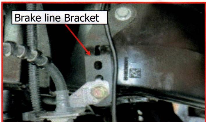
Gently pull the metal brake line down while lining up the brake line to the new bracket using the supplied **5/16" x 3/4" bolts, washers, and nuts**.
