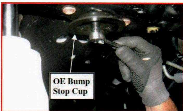
Install the **OE** bump stop cup to the bump stop extension using the supplied 8mm nut and washer.
