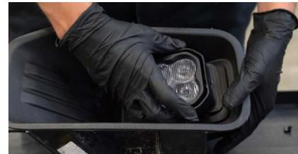
9. Install the SS3 bracket on to the factory bezel by flexing the retainer clips on the bezel as required.
