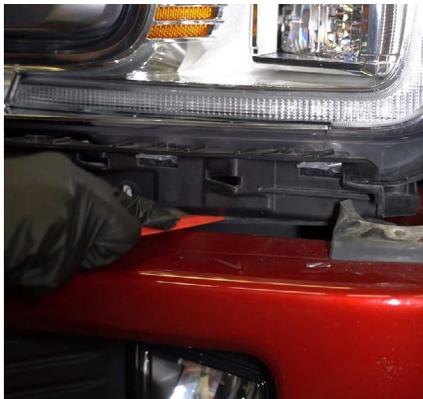
5. Remove the shroud blocking access to the fog light bezel. To do so, remove the 10mm bolt and loosen the three plastic pins holding it in place to the bottom of the headlight. Then remove the two 10mm bolts near the fender flare. Remove the shroud from the vehicle.
