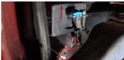
6. Remove the fog light bezel from the bumper, by removing the three 8mm bolts holding it in place and disconnecting the fog light harness. If applicable, remove the two 13mm bolts holding the bracket blocking the fog light bezel in order to gain access to the fog light bezel.
