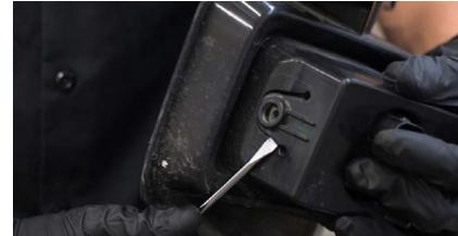
8. Remove the fog light housing from the bezel. To do so, remove the adjustment screw and spring from the fog light housing. Remove the factory fog light housing by prying up on the retainer clips holding it in place.
