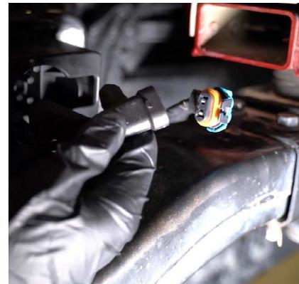
10. Reinstall the factory fog light bezel, by reinstalling the factory hardware. Plug the SS3 into the factory fog light harness using the included DT wire adapter. Test function. If the light does not turn on, try flipping the connector 180°.
