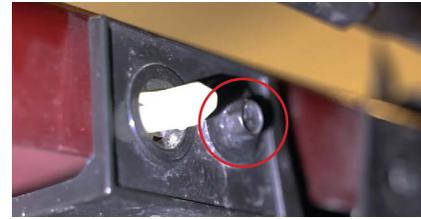
7. Remove the final 8mm bolt and loosen the plastic retaining clip to remove the fog light bezel from the vehicle.
