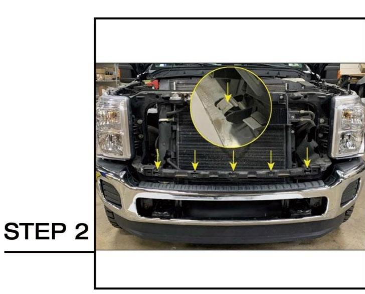
Gently pull the top of the grille away from the radiator support to gain access to the lower grille clips. Using a flathead screwdriver, press the top of the (5) mounting clips to dislodge the clips from thevehicle retainer panel. Once the (5) clips are depressed, remove the grille from the vehicle.
