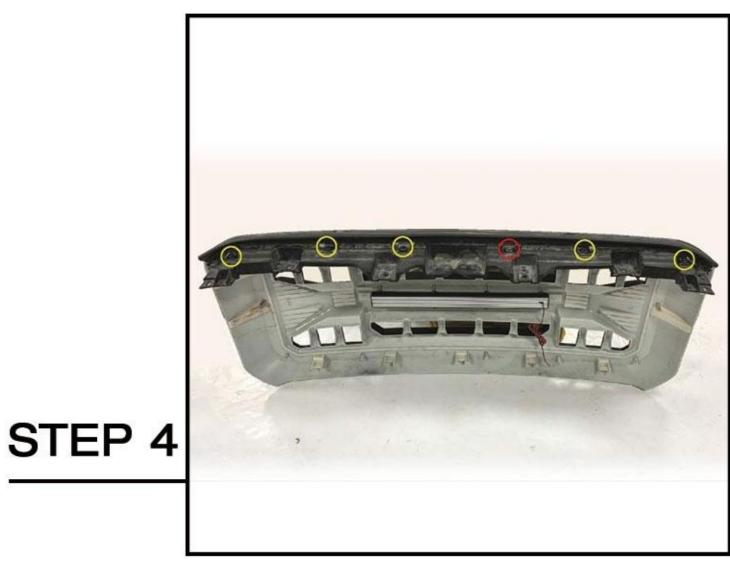
Transfer the upper grille shroud to the new grille reusing the original mounting hardware.
