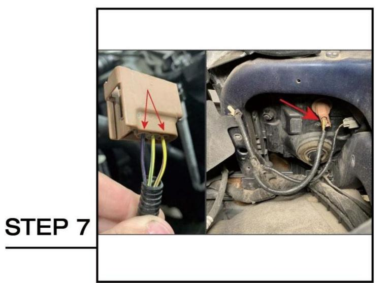
On the vehicle passenger side headlight assembly, locate the parking lamp/turn signal connector. Unplug the connector by pressing the tab to gain better access to the harness. Tap the LED light wiring into the vehicle parking light using the
