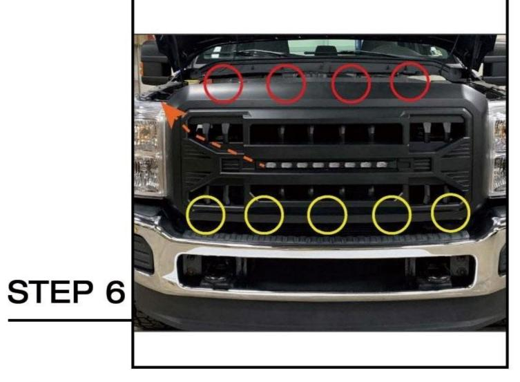
While routing the attached wiring harness away from the grille mounting points, fit the grille to the vehicle. Secure the lower clips first, then secure the top of the grille to the radiator support using the original (4)10mm bolts. Tighten all bolts evenly until secure. Route the LED wiring harness towards the vehicle passenger side headlight assembly.
