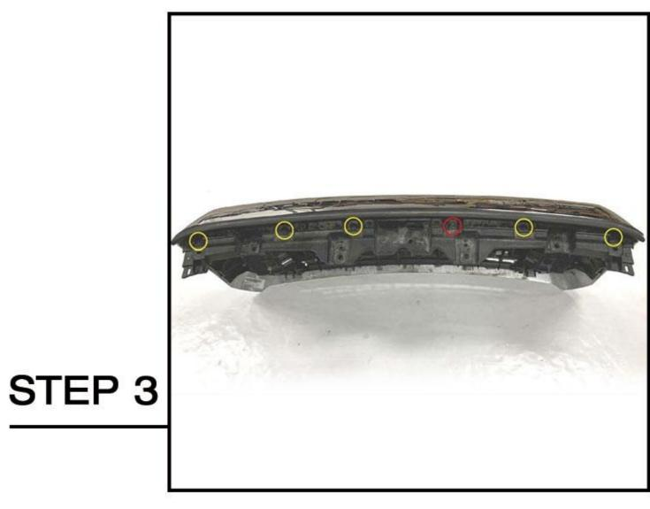
Remove (5) plastic push clips and (1) 10mm bolt to remove the upper grille shroud from the original vehicle grille. Note: The hardware will be reused.
