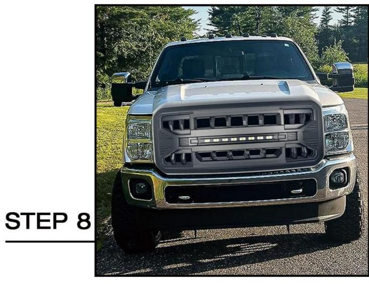
Close the vehicle hood and check the hood to grille alignment. If necessary, loosen the upper (4)10mm bolts to allow the top of the grille to adjust inward/outward. Adjust the grille until the hood and grille have a even gap across the top. Installation is now complete.
