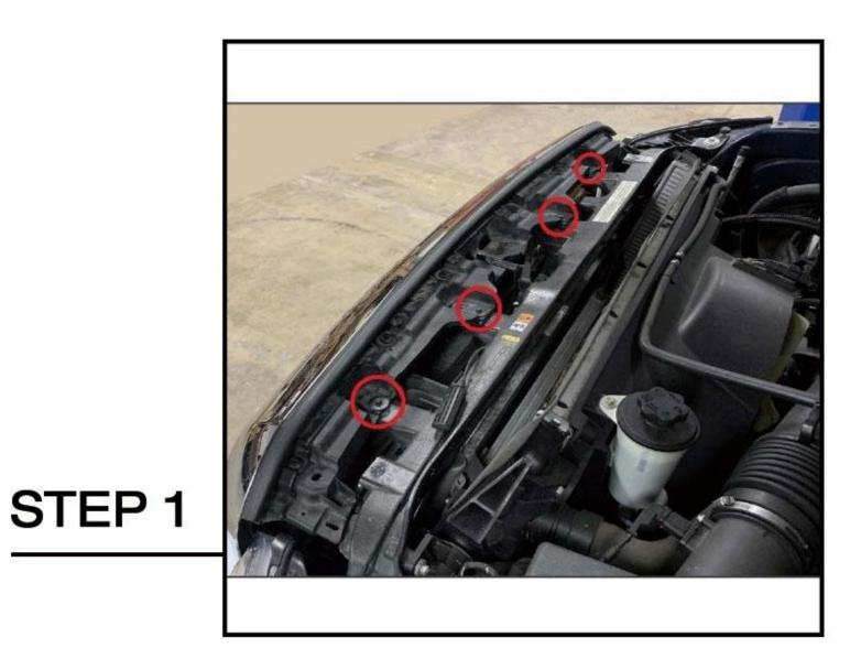
Open the vehicle hood. Locate the (4) 10mm bolts securing the top of the grille to the radiator support. Remove the (4) 10mm bolts.
