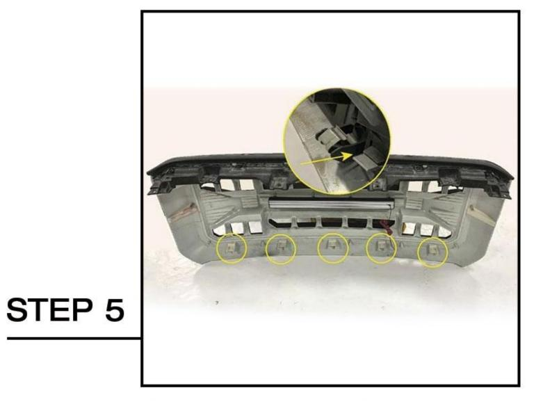
Install the (5) lower retaining clips to the vehicle grille.
