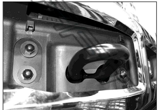
**(Fig 4) Remove bumper bolts (driver side pictured)**
