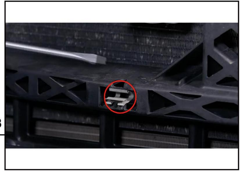
Pop the hood, remove 14 push tabs on the top with a pry tool, then grab this plastic piece and set it aside.
