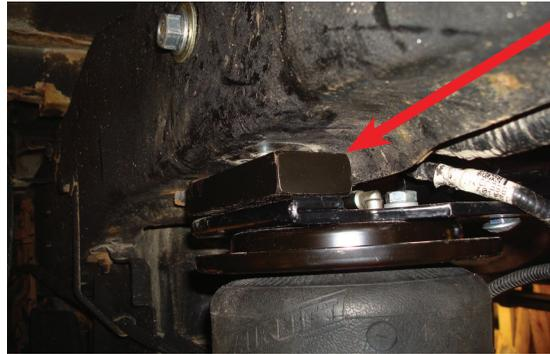
The spacer must be parallel to the frame with the wide portion facing out toward the wheel.
