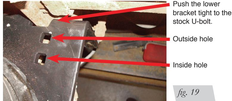
2. If installing this kit on a single-rear-wheel (SRW) vehicle, use the inside position square holes in the lower bracket to insert the long 3/8"-16 x 10" carriage bolts (Q) through (Fig. 19). If installing this kit on a dual-rear-wheel (DRW) vehicle, use the outside set of holes to insert the carriage bolts through.
