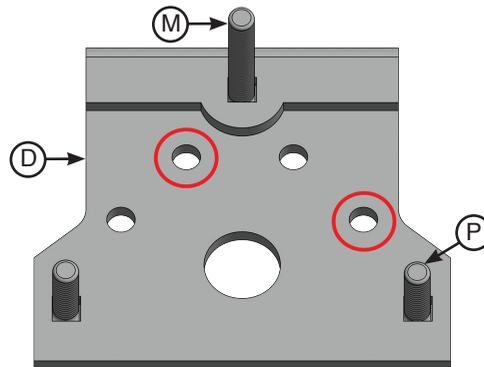
Passenger's (right) side installation mounting holes noted.
