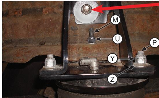
Torque both sides to 44 lb.-ft. (60Nm).
