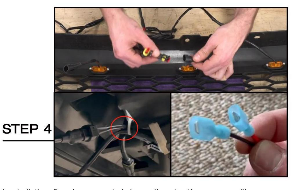
Install the five lower retaining clips to the new grille. Connect each amber light to the wiring harness and tie it up. Crimp the male spade connectors onto the positive and negative.
