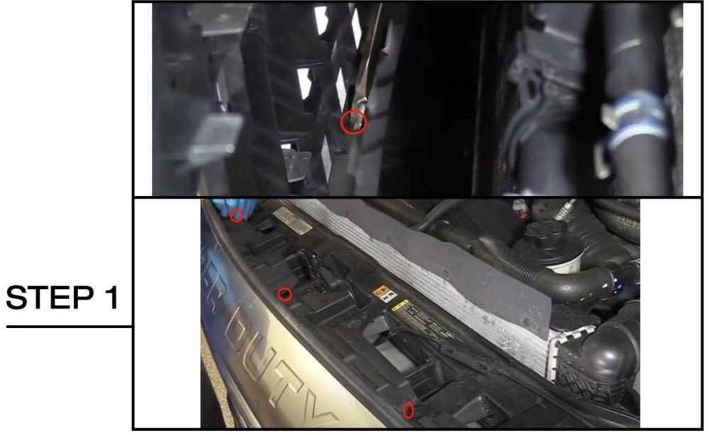
Open the hood, remove four 10-millimeter bolts along the
