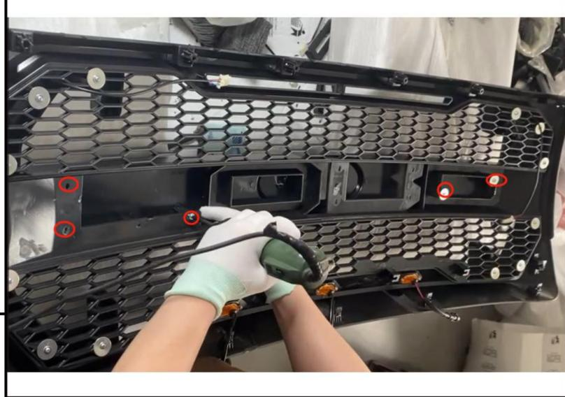
Remove five plastic push clips and one 10-millimeter bolt to remove the upper grille shroud from the original grille.
