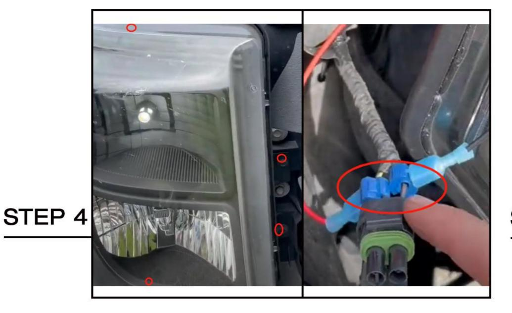
Remove 4 bolts to disconnect the headlight, place T-taps on the positive and negative wires of the headlights separately, then plug the red wire of the grille into the positive wire of the headlight and black to the negative wire. Reinstall the headlight.
