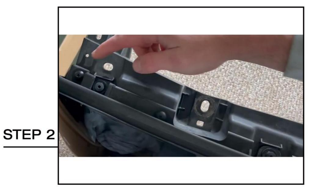
Remove five plastic push clips and one 10-millimeter bolt to remove the upper grille shroud from the original grille. (The hardware will be reused). Transfer the upper grille shroud to the new grille with the original mounting hardware.
