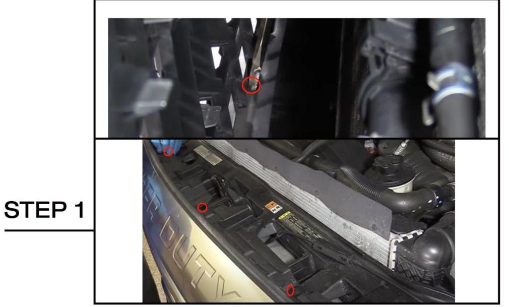
Open the hood,remove four 10-millimeter bolts along the top of the grille. Carefully lean the grille forward and locate the metal clips at the bottom, use a long flat blade screwdriver to push down and release these five clips. Then pull the grille off the truck.
