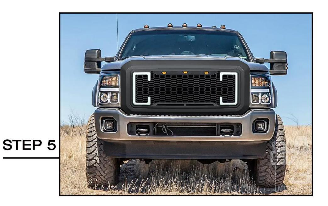
Connect daytime running lights with wiring harness that has two white connectors. Then connect the red wire to the ACC, the black wire to the negative of battery, the yellow wire connects to the turn signal. Align the grille with the clips at the bottom, press hard. Follow the step 1 in reverse order to install the new grille to complete the installation.
