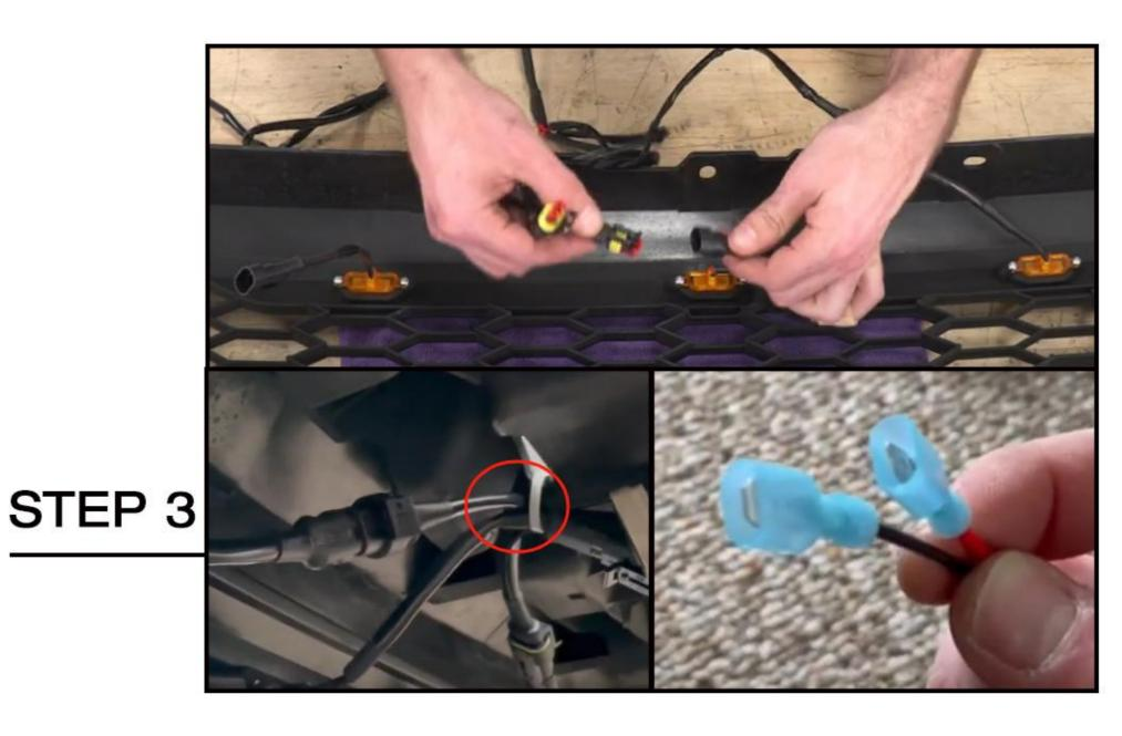
Install the five lower retaining clips to the new grille. Connect each amber light to the wiring harness and tie it up. Crimp the male spade connectors onto the positive and negative.
