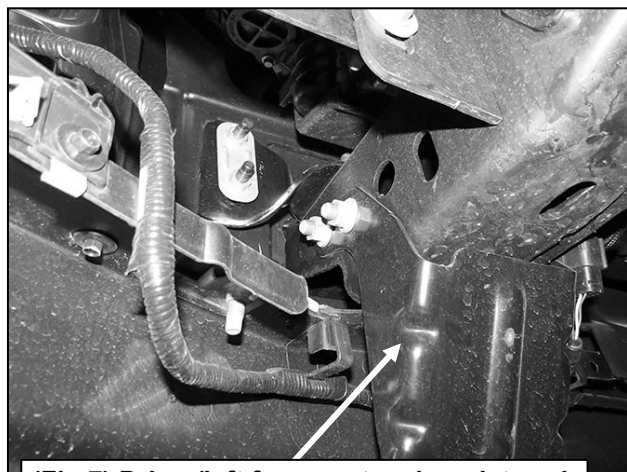
(Fig 7) Driver/left frame extension pictured
