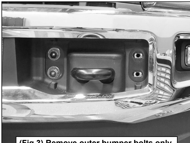
(Fig 3) Remove outer bumper bolts only
