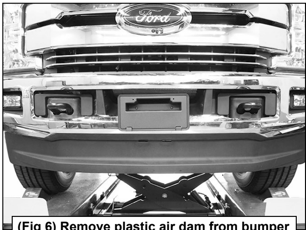
(Fig 6) Remove plastic air dam from bumper
