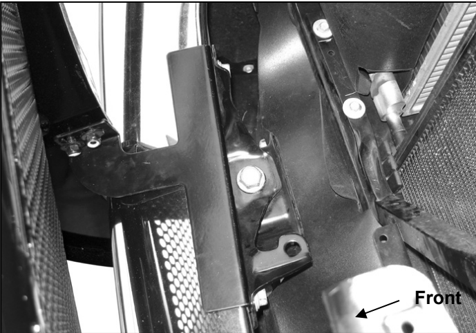
(Fig 10) Passenger side Top Bracket installation pictured from above
