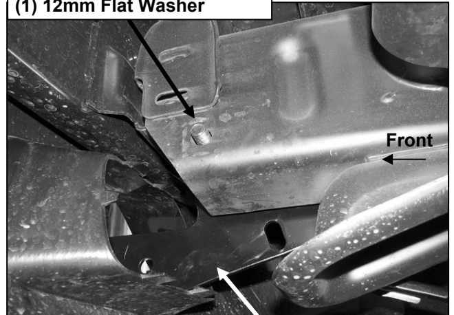
(Fig 4) Passenger side Mounting Bracket pictured
