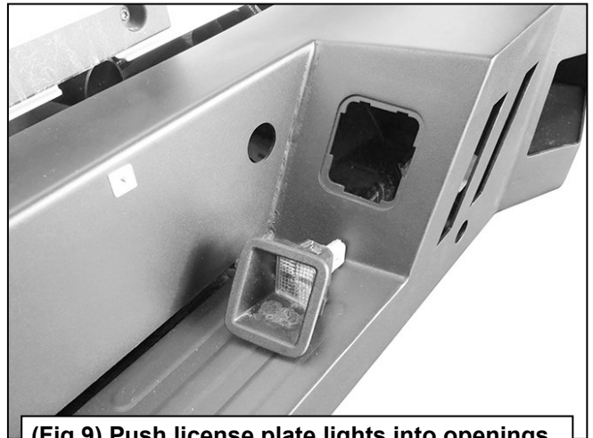
(Fig 9) Push license plate lights into openings
