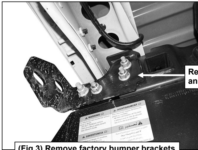
(Fig 3) Remove factory bumper brackets
