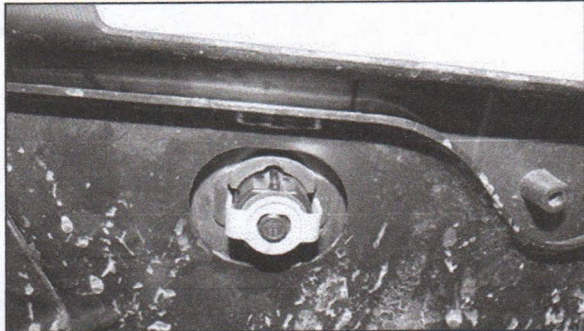
(Fig 12) Remove sensors, wire harness, license plate lights, trailer plug and spare tire access lock (pictured) if equipped
