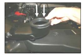
**6.** Re-install the rubber seal removed in step #3 onto the Airaid Intake Tube. Use caution to align the notch in the tube with the notch in the seal.
