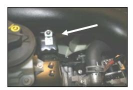
**16.** Install the L-shaped bracket (#25) using one ½ -20 x 1/2" button head bolt (#14) and 1/4" flat washer (#15) thru the oval slot into the backside of the tube. Next, install one 6mm bolt (#16) and 1/4" flat washer (#15) thru the round hole into the factory bracket. Tighten the hose clamps on the hump hose. Some adjustment of the factory bracket may be necessary for a proper fit, see step #17.
