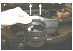
**3.** Remove the rubber seal from the factory airbox and save it for re-installation in step #6.
