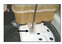
**11.** Using a 5/16" socket, remove one bolt from the factory coolant reservoir mount.
