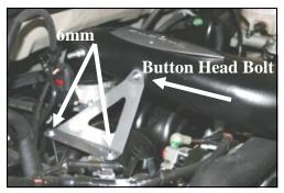
14. Install the two brackets (#7, #8) from the Airaid Intake tube onto the intake manifold using two  $\frac{1}{4}$  -20 x  $\frac{1}{2}$ " button head bolts (#14), and 1/4" flat washers (#15) on the tube, and four 6mm bolts (#16), and 1/4" flat washers (#15) on the bottom. Leave the button head bolts loose for now.
