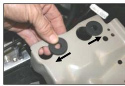
**8.** Slip two rubber grommets (#22) into the large holes in the bracket on the drivers side fender, then slide them sideways into the smaller holes as shown.
