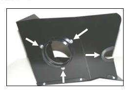
**10.** Install the air filter adapter (#2) into the **CAD** using three  $\frac{1}{4}$  - 20 x  $\frac{1}{2}$ " button head bolts (#14) and  $\frac{1}{4}$ " flat washers (#15). Next, install the 4" rubber trim (#23), as shown.
