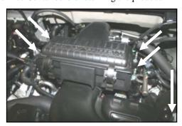
**2.** Using a 10mm deep socket, remove the 4 tower bolts, two on each side of the factory airbox. Remove one bolt holding the factory intake tube to the mounting bracket. Remove the complete factory intake system.
