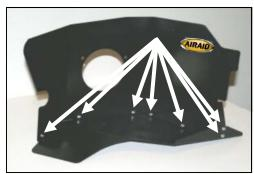
**9.** Assemble the two Cool Air Dam (CAD) panels (#3, #4) using seven 6-32 x 5/16' screws (#11), #6 flat washers (#12), and 6-32 keps nuts (#13). Apply the Airaid Decal as shown.
