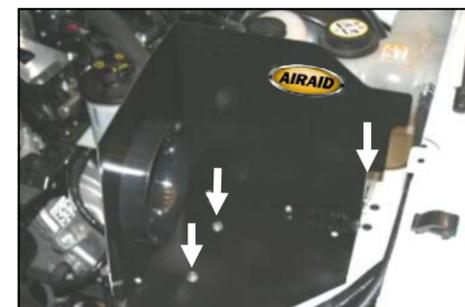
12. Install the CAD into the vehicle with one 6mm bolt (#16) and 1/4" flat washer (#15) through the panel, through the coolant reservoir mount and into the speed nut below it. Using two 6mm bolts (#16) two 1/4" flat washers (#15), two 1/4" lock washers (#17), and two M6 hex nuts (#18), insert the two bolts thru the CAD, thru the grommets, and thru the long/narrow bracket (#19). Use the line drawing above for reference.
