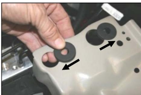
8. Slip two rubber grommets (#22) into the large holes in the bracket on the drivers side fender, then slide them sideways into the smaller holes as shown.
