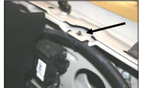
18. Slip the black plastic hose mount (#26) over the radiator overflow hose. Next, place one 1/4" flat washer (#15) over the hole on the inner drivers side fender. Slide the hose mount prongs thru the fender and thru the washer.
