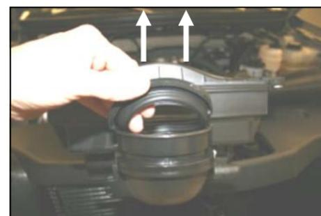
3. Remove the rubber seal from the factory airbox and save it for re-installation in step #6.
