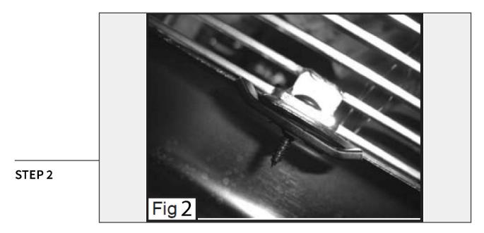
Using the provided clip nuts and brackets, fit the clip nuts around the bracket and align the clip nut screw hole to the bracket hole. Then, fit the included Phillips screws through the grille panel bolt holes as well as the bumper bolt holes, and thread the Phillips screw into the clip nuts/bracket assembly.
