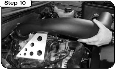
Place urethane coupler on the throttle body (see diagram below for correct coupler position) and the housing. Position intake duct into engine bay and tighten down the clamps.
