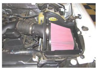
**13.** Install the Airaid Premium Filter (#1) on to the Air Meter Tube and tighten the clamp.
