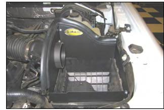
**12.** Install the Weather Strip (#5) to the Panel assembly as shown, with the contour rolling away from the filter
