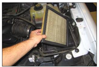
4. Remove the Factory air filter.
