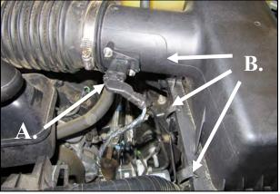
2. A. Disconnect the Air meter in the factory airbox
