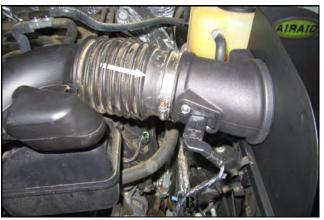
**11.** Slide the factory intake tube onto the Airaid Tube and tighten the clamp. Reconnect the Mass Air Flow sensor.
