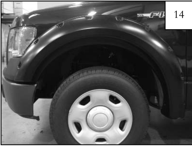
Completed front flare installation.
