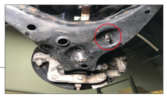
Using a 18mm socket, remove the nut securing the sway bar end link to the lower control arm.
