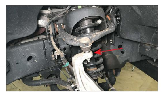
Using a 18mm socket, loosen the nut securing the upper ball joint to the knuckle. Using a hammer, strike the knuckle to separate the ball joint from the knuckle. Remove the nut to separate the control arm from the knuckle. This will allow additional space when removing the strut assembly from the vehicle.
