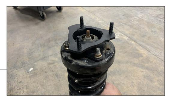
Secure the included strut spacer to the top of the vehicle strut using the included (3) M10 flange nuts. Tighten the nuts to 52 ft. lbs.
