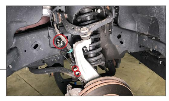
Begin by safely lifting and supporting the front of the vehicle with a jack and jack stands. Using a 22mm socket or lug nut socket, remove the front wheels.
