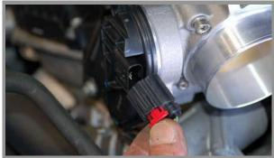
Using the supplied bolts, install the BBK throttle body onto the intake manifold and tighten the bolts. Reconnect the electrical connection.
