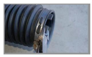
• The stock air inlet tube will work with the BBK throttle body. Just open the clamp all the way up before installing. Trim off the 2 small tabs on the top of the stock rubber inlet tube so it will fit all the way onto the BBK throttle body. A little WD-40 or light grease may help this process.
