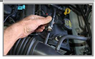
Disconnect the (2) breather hoses attached to the inlet tube.
