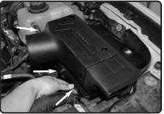
**10.** Install the Injen upper airbox and plenum onto the lower OEM airbox assembly and attach the 3 factory metal clips to secure the Injen air box to the OEM air box
