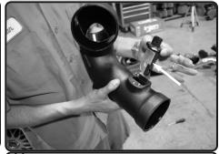
11. Place the MAF sensor into the Injen intake tube and secure it with the two M4 supplied screws.
