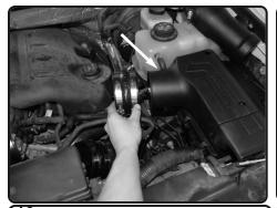
**13.** Place the 4.00" hump hose and 2-#64 clamps onto the Injen intake plenum. Make sure you push the hump hose all the way over to allow room for the intake tube.
