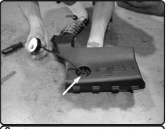
**6.** Place the grommet into the Injen upper air box. Next, connect the 3mm vacuum line to the Filter Minder. Then insert the vacuum line through the grommet.
