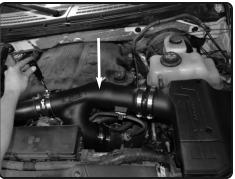
**15.** Install the Injen intake tube and connect all the couplers and secure the intake tube by tightening the clamps once its been adjusted.
