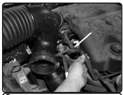
**5.** If your vehicle is equipped with with a vacuum line, disconnect it and place to the side for now.
