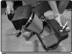
**7.** Once the Filter Minder is installed in the upper air box, install the filter onto the Injen air box plenum.
