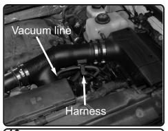
**16.** Connect the vacuum line to the 3/8" barbed fitting if equipped and then connect the MAF sensor harness to the MAF sensor.
