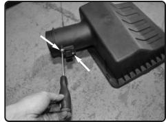
Remove the two torq screws and remove the MAF sensor from the upper air box assembly
