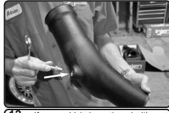
**12.** If your vehicle is equipped with a vacuum line, place the 1/4 NPT 3/8 barbed fitting into the insert on the intake tube. Place the 1/4 NPT plug if no vacuum line is present
