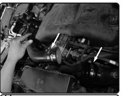
**14.** Place a 4.00" humpse and 2-#64 clamps onto the 4.00" OE inlet tube and the 3.50"-3.25" step hose and #48 & # 56 clamp onto the 3.25" OE inlet tube.
