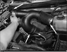
**4.** Loosen the three clamps on the factory Y-air duct and remove it from the engine bay.
