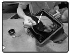
**9.** Connect the 3mm vacuum line from the filter minder in figure 6 to the fitting on top of the filter.
