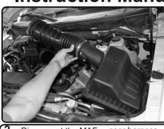
**2.** Disconnect the MAF sensor harness and unclip the 3 metal tabs holding the upper air box to the lower air box. Loosen the clamp on the air duct and then remove the upper box assembly and air filter panel.
