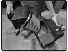
**5.** Once the Filter Minder is installed in the upper air box, install the filter onto the Injen air box plenum.
