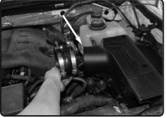
**9.** Place the 4.00" hump hose and 2-#64 clamps onto the Injen intake plenum. Make sure you push the hump hose all the way over to allow room for the intake tube. Page 3 EVO9101
