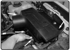
**8.** Install the Injen upper airbox and plenum onto the lower OEM airbox assembly and attach the 3 factory metal clips to secure the Injen air box to the OEM air box
