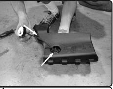
**4.** Place the grommet into the Injen upper air box. Next, connect the 3mm vacuum line to the Filter Minder. Then insert the vacuum line through the grommet.
