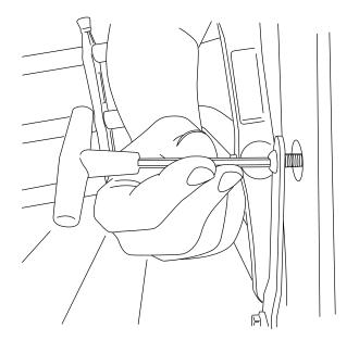
Repeat for lower hole. Torque to 22 ft.lbs. Repeat steps 1-8 for vehicles without bedliner and steps 9-14 for vehicles with bedliner on other side.
