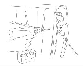
Verify that the holes are large enough and align with the factory bed pillar holes.
