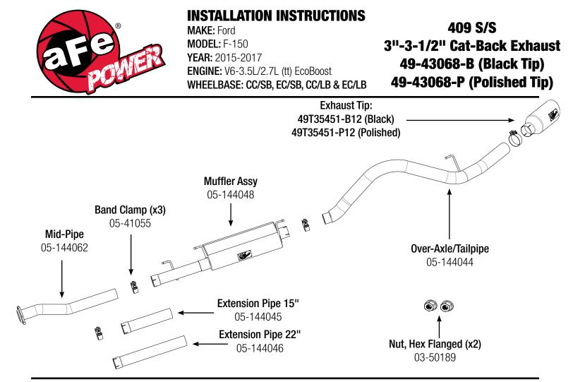
Step 1: (Read Instructions prior to installation) Remove your stock exhaust up to the catalytic converter from the rear of your truck, working your way forward. Take caution not to damage the factory hardware and isolation mounts as they will be reused. (it is recommended to not fully tighten the clamps until the entire system has been installed.)
