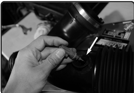
8. Loosen and remove the temperature sensor out of stock intake. Use a small flat head screwdriver to pull back clip on sensor.
