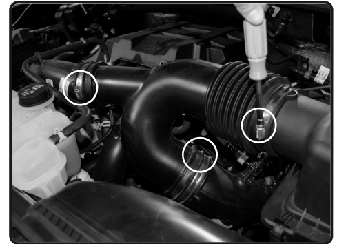
3. Loosen the 3 clamps on the stock intake tube using 7mm nut driver.
