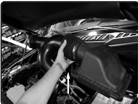
4. Un-clip the upper half of the air box attached to bottom of air box. Remove stock assembly out of vehicle.
