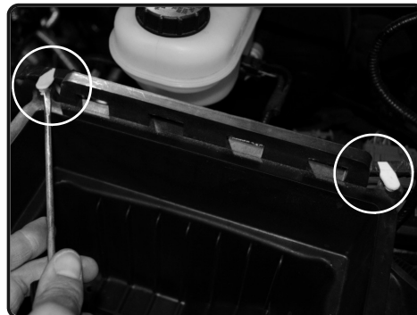
6. Pull back the temperature harness from the air box.
